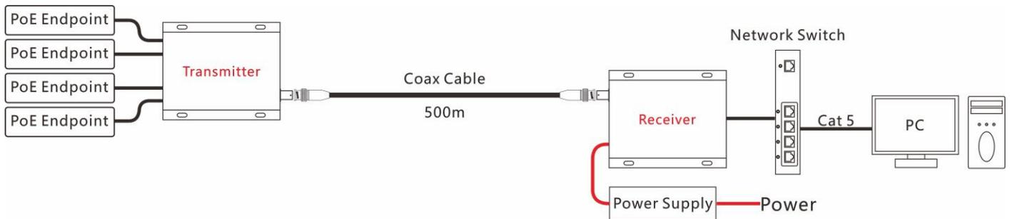
2. When the Receiver unit is powered by a PoE switch, both the Transmitter unit and PoE devices are powered without requiring an external power supply.
