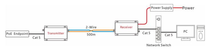
2. Provide low voltage 12VDC output for front-end IP Endpoint.
